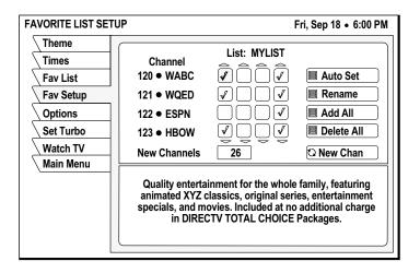
The four columns of small boxes on the right hand side of the pane are the *Tag Boxes*. The first three columns are the *Fav.A*, *Fav.B*, and *Fav.C*. channel lists. The farthest right hand column is the *Family* list.
